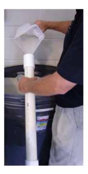
5) Take ½ in pvc pipe and attach it to the 2in pvc pipe using the glue.
